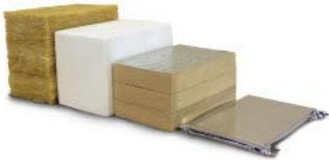
NanoPore insulation, shown on the right in its vacuum packaging, provides insulation of R-40 per inch with a material containing 30–50 nanometer pores, ideal for preventing conduction of heat. The insulation provides the same R-value as the thickness of fiberglass, expanded polystyrene, and polyisocyanurate foam shown, respectively.
