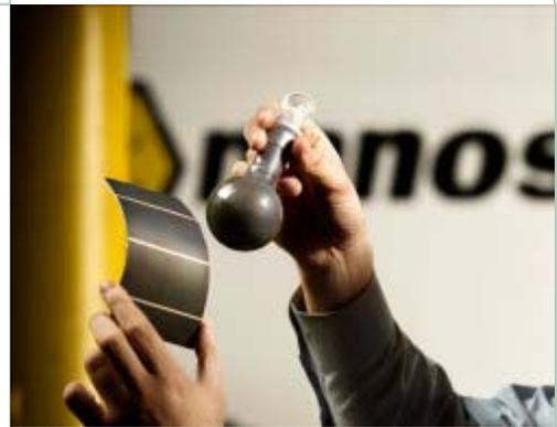
Using an “ink” that includes nanoparticles, materials the size of a billionth of a meter, Nanosolar “prints” thin-film solar photovoltaic cells on a foil substrate. The particles self-assemble into a semiconductor that drives electricity production.
