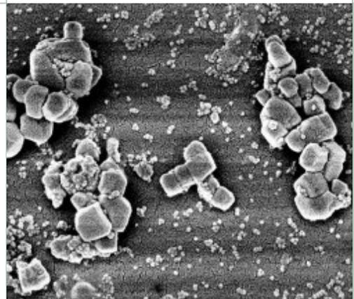
This electron-microscope image shows the Greenshield texture finish with silica and flouorocarbon nanoparticles bonded to fabric.
